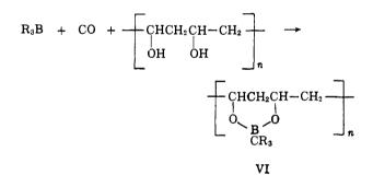
The polymer could be cast into transparent colorless films and drawn into fibers.
